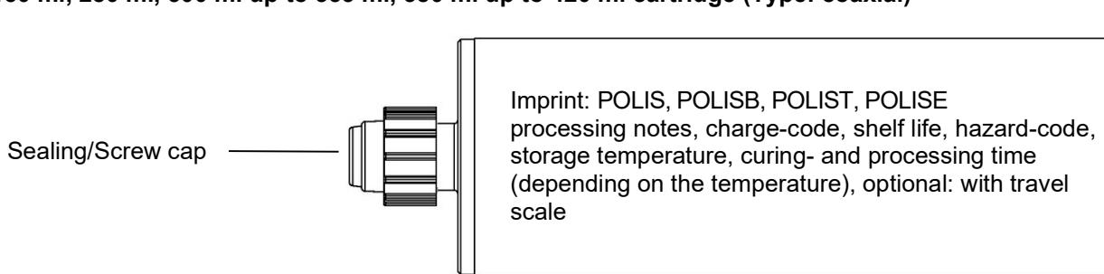
**235 ml, 345 ml up to 360 ml, 825 ml cartridge (Type: "side-by-side")**
