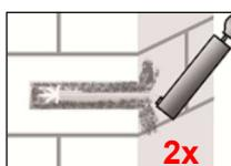
3. Holes to be drilled perpendicular to the surface of the base material by using a hard-metal tipped hammer drill bit. Drill a hole, with drill method according to Annex C4 – C39, into the base material, with nominal drill hole diameter and bore hole depth acc. to the size and embedment depth required by the selected anchor. In case of aborted drill hole the drill hole shall be filled with mortar.
