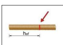
6. The position of the embedment depth shall be marked on the threaded rod. Push the threaded rod into the drill hole while turning slightly to ensure positive distribution of the adhesive until the embedment depth is reached. The anchor shall be free of dirt, grease, oil or other foreign material.
