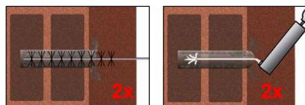
4. Blow out from the bottom of the drill hole two times. Attach the appropriate sized brush ( $> d_{b,min}$  Table B2 or B3) to a drilling machine or a battery screwdriver, brush the hole clean two times, and finally blow out the hole again two times.
