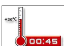
8. Allow the adhesive to cure to the specified time prior to applying any load or torque. Do not move or load the anchor until it is fully cured (attend Table B4).
