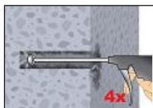
**After cleaning, the bore hole has to be protected against re-contamination in an appropriate way, until dispensing the mortar in the bore hole. If necessary, the cleaning repeated has to be directly before dispensing the mortar.**
