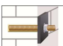
9. After full curing, the fixture can be installed with up to the max. torque (see parameters of brick Annex C5 to Annex C39) by using a calibrated torque wrench.
