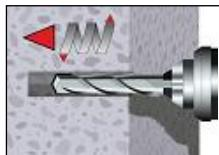
1. Drill with hammer drill a hole into the base material to the size and embedment depth required by the selected anchor (Table B1). In case of aborted drill hole: the drill hole shall be filled with mortar.
