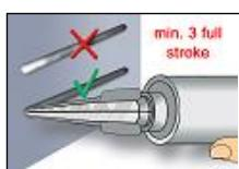
5. Prior to dispensing into the drill hole, squeeze out separately a minimum of three full strokes and discard non-uniformly mixed adhesive components until the mortar shows a consistent grey or blue (POLISB) colour. For foil tube cartridges it must be discarded a minimum of six full strokes.
