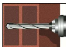
3. Holes to be drilled perpendicular to the surface of the base material by using a hard-metal tipped hammer drill bit. Drill a hole, with drill method according to Annex C4 – C39, into the base material, with nominal drill hole diameter and drill hole depth acc. to the size and embedment depth required by the selected anchor. In case of aborted drill hole the drill hole shall be filled with mortar.
