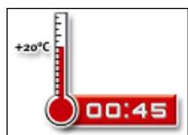
8. Allow the adhesive to cure to the specified curing time prior to applying any load or torque. Do not move or load the anchor until it is fully cured (attend Table B4).
