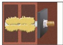
9. After full curing, the fixture can be installed with up to the max. torque (see parameters of brick Annex C5 to Annex C39) by using a calibrated torque wrench.
