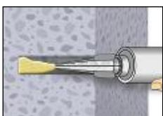
**6.** Starting from the bottom or back of the cleaned anchor hole fill the hole up to approximately two-thirds with adhesive. Slowly withdraw the static mixing nozzle as the hole fills to avoid creating air pockets. If the bottom or back of the anchor hole is not reached, an appropriate extension nozzle must be used. Observe the gel-/ working times given in Table B3.
