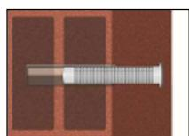
5. Insert the sleeve flush with the surface of the masonry. Only use sleeves that have the right length. Never cut the sleeve except the sleeve 16x130/330. For installing the sleeve 16x130/330 measure the required length of sleeve, cut the sleeve from the top and set the cap on it before pushing it through the fixing element.
