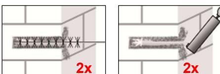
4. Blow out from the bottom of the drill hole two times. Attach the appropriate sized brush ( $> d_{b,min}$  Table B2 or B3) to a drilling machine or a battery screwdriver, brush the hole clean two times, and finally blow out the hole again two times.
