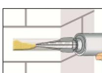
5. Starting from the bottom or back of the cleaned anchor hole fill the hole up to approximately two-thirds with adhesive. Slowly withdraw the static mixing nozzle as the hole fills to avoid creating air pockets.
