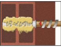
7. The position of the embedment depth shall be marked on the threaded rod. Push the threaded rod into the drill hole while turning slightly to ensure positive distribution of the adhesive until the embedment depth is reached. The anchor shall be free of dirt, grease, oil or other foreign material.
