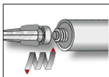
3. Attach a supplied static-mixing nozzle to the cartridge and load the cartridge into the correct dispensing tool. Cut off the foil tube clip before use.
