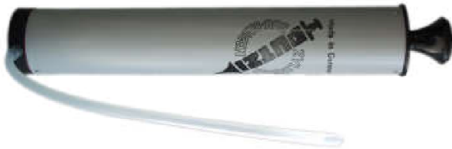
MAC - Hand pump (volume 750 ml) Drill bit diameter ( d_0 ): 10 mm to 20 mm Drill hole depth ( h_0 ): < 10 d_{nom} Only in uncracked concrete
